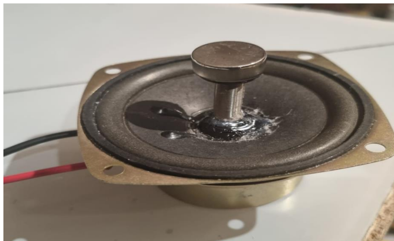
Spring Mass System with Base Excitation
